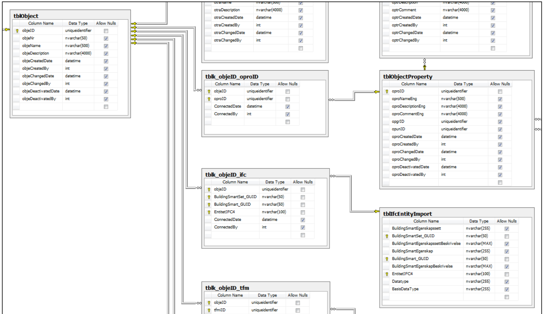
ER-extract showing the relationship between an object (i.e. product) and its mapping to an IFC-entity (imported entities)
